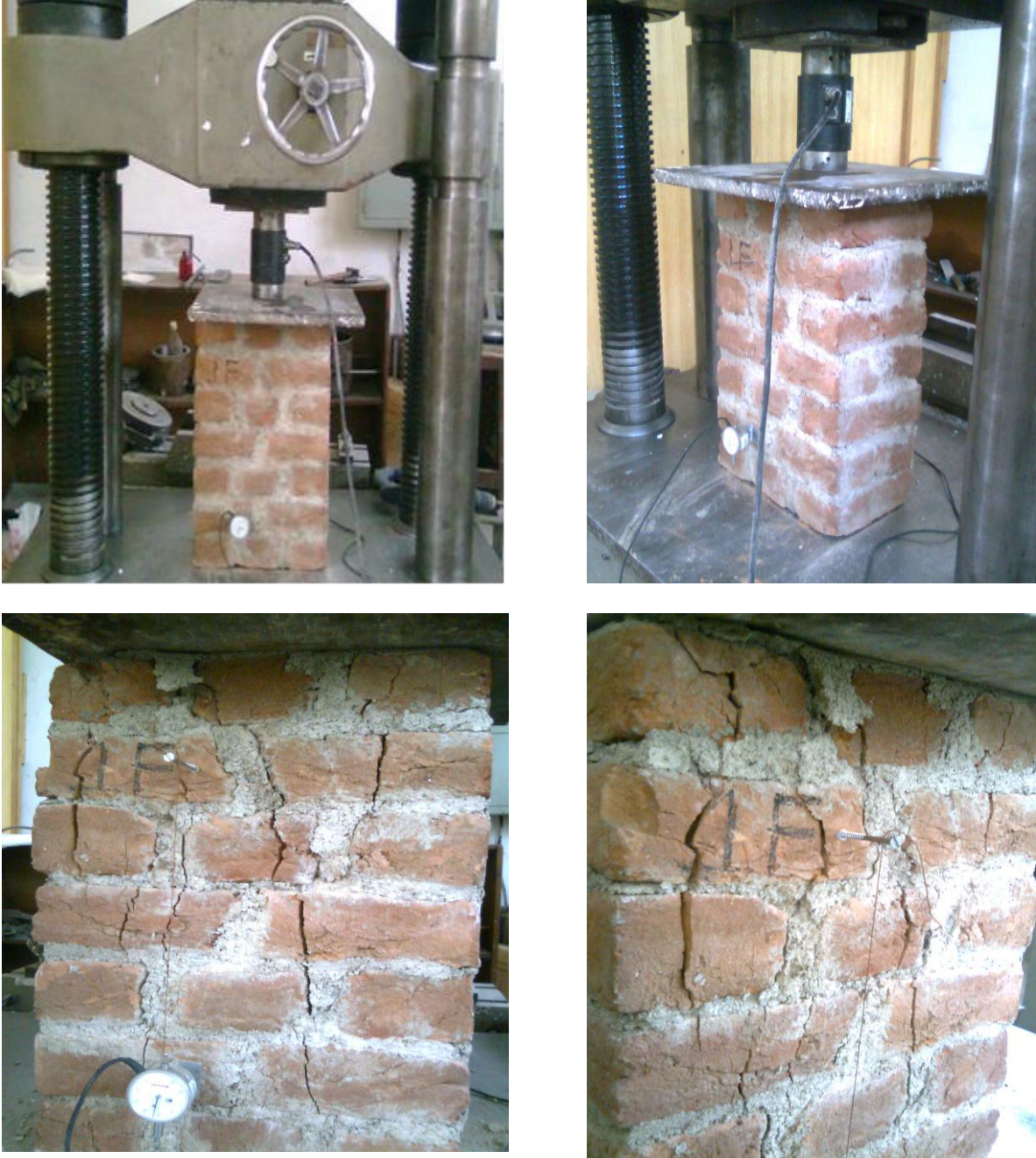
Figure 2: Testing of Masonry Assemblage
