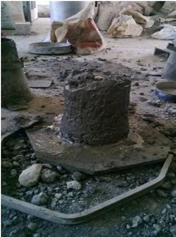
Fig 5.1(a) Slump Test of CS
