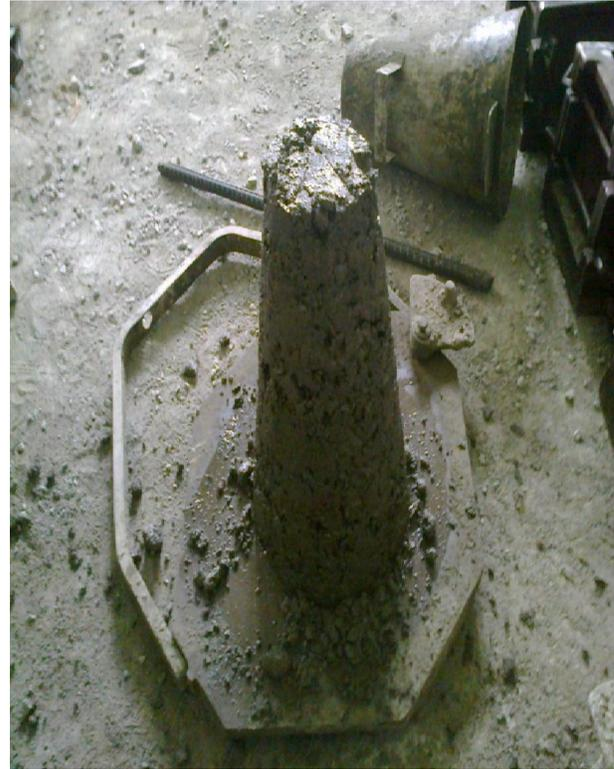
Fig 5.1(b) Slump Test of PRS
