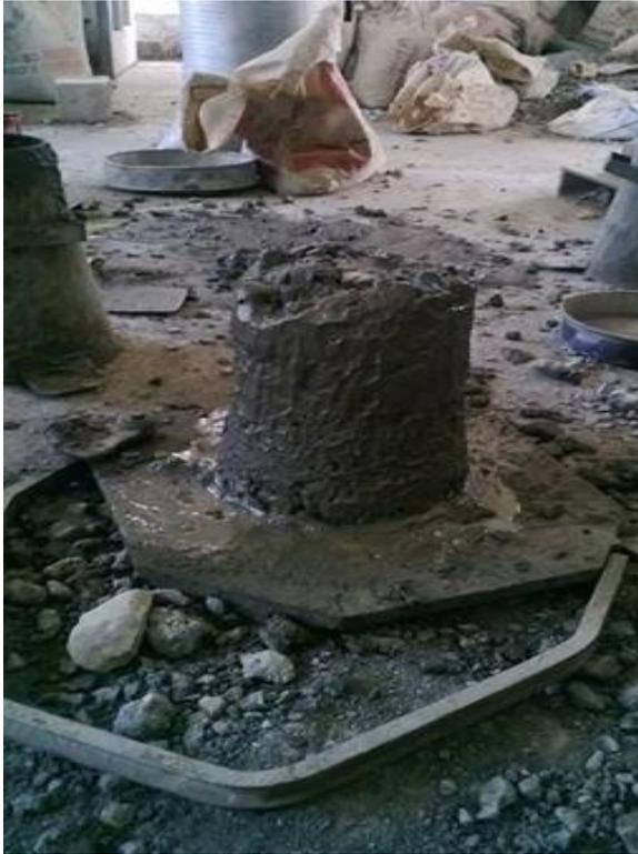
Fig 5.1(a) Slump Test of CS
