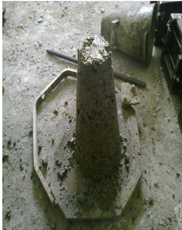
Fig 5.1(b) Slump Test of PRS
