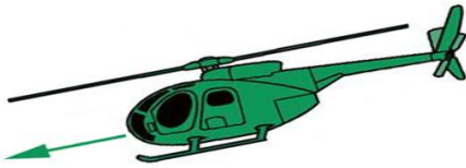
Fig 2(c): Lateral cyclic pitch control
